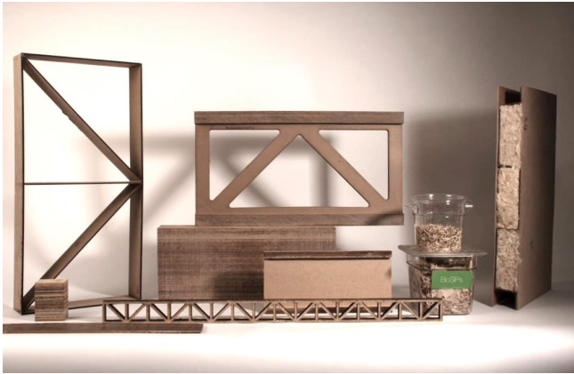
Figure 1. BioSIPS Low Life Cycle Analysis structural inventions from 100% cellulose waste fibers. Image Credit: Julee Herdt.
